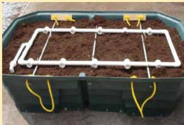
**Some onlot disposal systems require effluent to pass through a filtration unit before it is dispersed to the absorption field. One option is a peat biofilter, which uses partially decomposed plant material to remove contaminants from the wastewater. (Photo courtesy of DEP.)**
